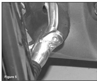
Remove the two bolts that secure the left foot peg bracket, figure 4. Mount the shift cylinder support bracket by inserting the supplied 8mm x 50mm socket head cap screws through the bracket from the Pingel logo side, followed by the supplied spacers (with taper pointing towards the motorcycle) and the stock footpeg bracket. Apply thread locker to the bolts and install the assembly to the motorcycle frame at the original footpeg location, holding the bracket forward while tightening.
